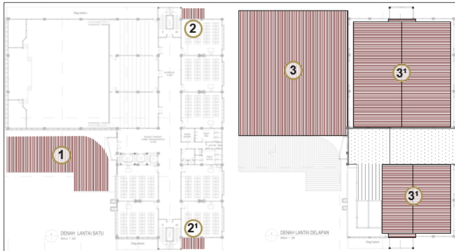
Figure 14. The area calculation for albedo on the rooftop of the Riau Polytechnic Tower (source: author)
