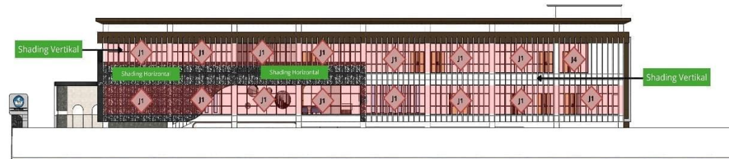
Figure 6. (d) Type of openings and shading on the east elevation (source: author, 2026)
