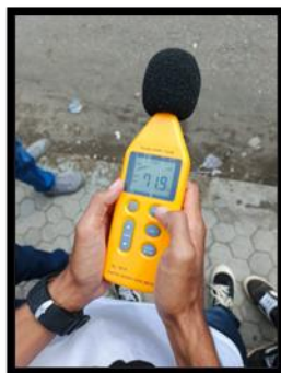
Figure 1. Sound Level Meter was used as the measuring device (source: author)
